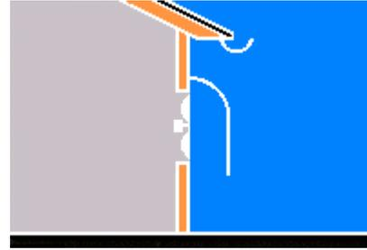
Good design - rounded, smooth interior, ground clearance and correct far width.
