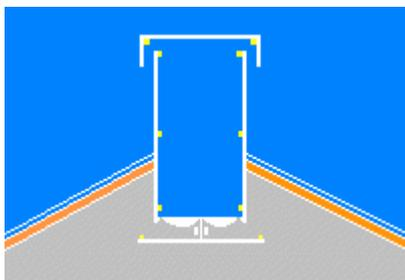
Poor design - international obstruction, square cap and turbulent airflow
