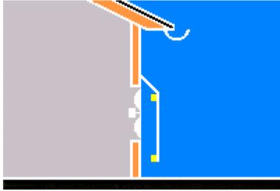
Poor design - obstructed interior, too near ground and too narrow.
